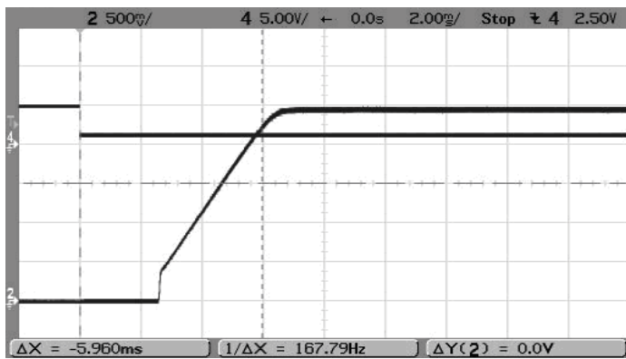
Step Load Transient Response (Vin=12V, Vout=2.5V, Cloud=0, Iout=1.5A to 3A) Trace 2=Vout, 100 mV/div. Trace 4=Iout, 2.5A/div.
