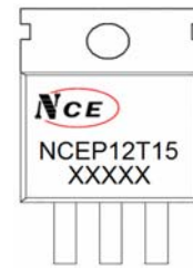
Marking and pin assignment
