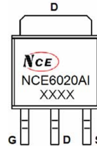
Marking and pin assignment
