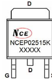
Marking and pin assignment
