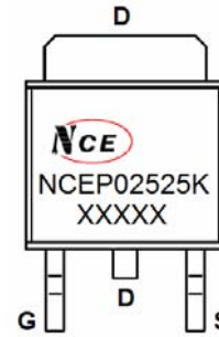
Marking and pin assignment
