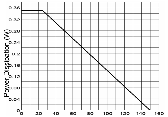
T_J -Junction Temperature( ^{\circ}\text{C} ) Figure 9 Power De-rating
