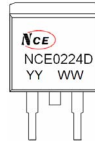
Marking and pin assignment
