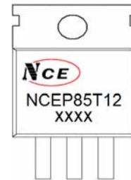
Marking and pin assignment
