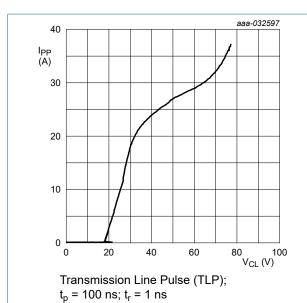
Fig. 6. Dynamic resistance with positive clamping; typical values
