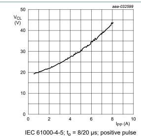
Fig. 8. Dynamic resistance with positive clamping; typical values
