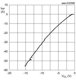
Transmission Line Pulse (TLP);  $t_p = 100 \text{ ns}$ ;  $t_r = 1 \text{ ns}$
