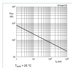
Fig. 3. Peak pulse power dissipation as a function of pulse duration; typical values
