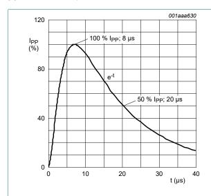
Fig. 1. 8/20 µs pulse waveform according to IEC 61000-4-5
