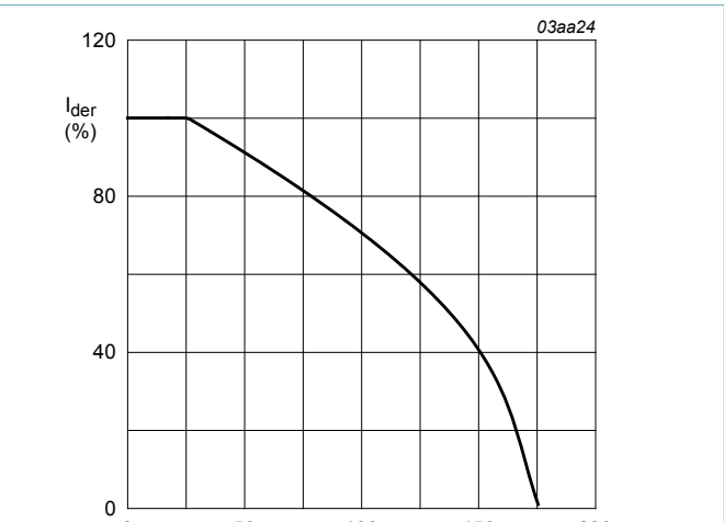
Fig. 2. Normalized continuous drain current as a function of mounting base temperature
