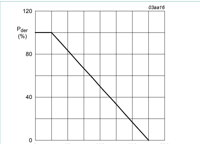
Fig. 1. Normalized total power dissipation as a function of mounting base temperature
