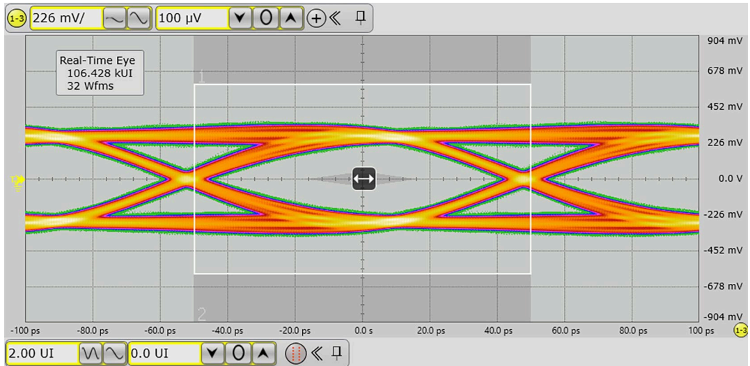
Fig. 5. USB3.2 eye diagram, PCB with device; typical values
