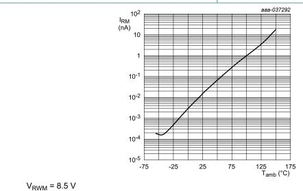
Fig. 7. Reverse leakage current as a function of ambient temperature; typical values
