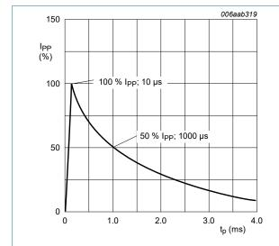
Fig. 1. 10/1000 µs pulse waveform according to IEC 61643-321
