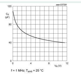
Fig. 6. Diode capacitance as a function of reverse voltage; typical values
