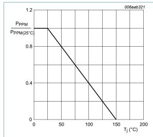
Fig. 3. Relative variation of rated peak pulse power as a function of junction temperature; typical values
