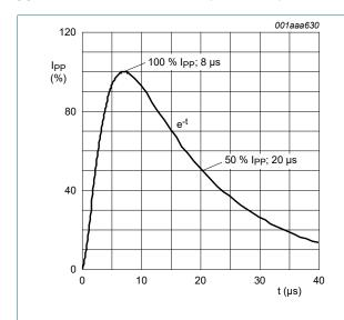
Fig. 2. 8/20 µs pulse waveform according to IEC 61000-4-5
