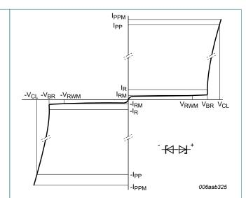
ig. 5. V-I characteristics for a bidirectional ESD protection diode
