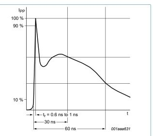
Fig. 3. ESD pulse waveform according to IEC 61000-4-2
