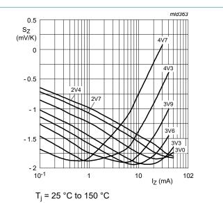
Fig. 2. Temperature coefficient as a function of working current; typical values (BZB784-C2V4 to C4V7)
