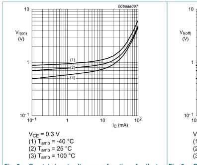
On-state input voltage as a function of collector | Fig. 6. Fig. 5. current; typical values
