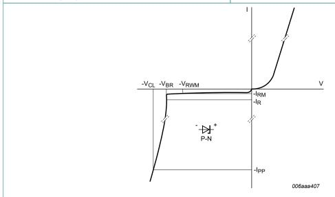
Fig. 6. V-I characteristics for a unidirectional ESD protection diode
