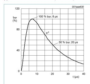
Fig. 1.  $8/20~\mu s$  pulse waveform according to IEC 61000-4-5
