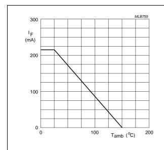
Device mounted on an FR4 printed-circuit board.
