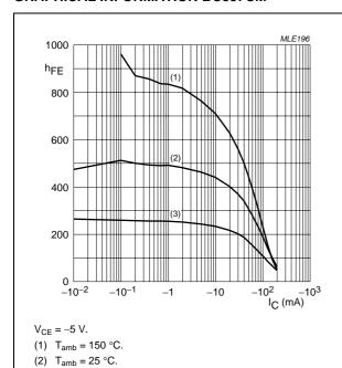
Fig.10 DC current gain; typical values.
