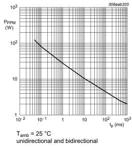
Fig. 3. Rated peak pulse power as a function of exponential pulse duration (rectangular waveform); typical values
