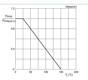
Relative variation of rated peak pulse power Fig. 4. as a function of junction temperature; typical values
