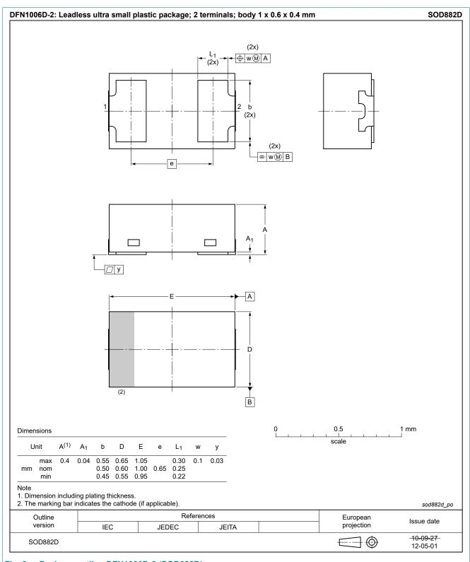
Fig. 8. Package outline DFN1006D-2 (SOD882D)
