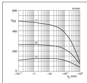
**TR2 (PNP)**  $V_{CE} = -2 \text{ V}.$
