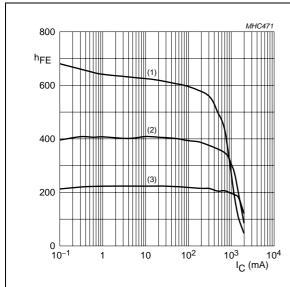
**TR1 (NPN);**  $V_{CE} = 5 \text{ V}.$
