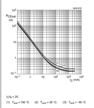
Fig.7 Collector-emitter equivalent on-resistance as a function of collector current; typical values.
