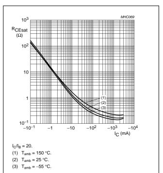
Fig.7 Equivalent on-resistance as a function of collector current; typical values.
