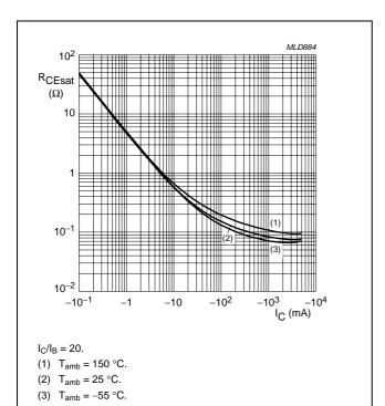
Fig.10 Equivalent on-resistance as a function of collector current; typical values.
