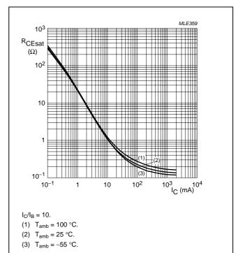
Fig.14 Collector-emitter equivalent on-resistance as a function of collector current; typical values.
