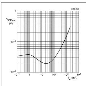
$I_{C}/I_{B} = 20.$  $T_{amb} = 25 \,^{\circ}C.$
