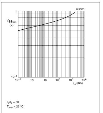
Fig.12 Base-emitter saturation voltage as a function of collector current; typical values.
