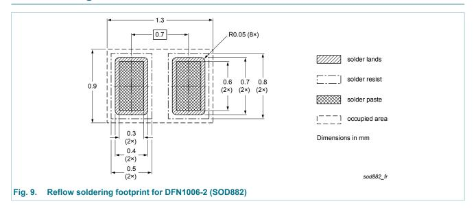
Ultra low capacitance bidirectional ESD protection diode
