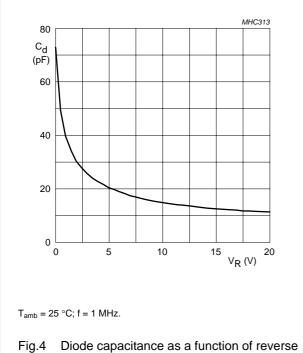
ig.4 Diode capacitance as a function of revers voltage; typical values.
