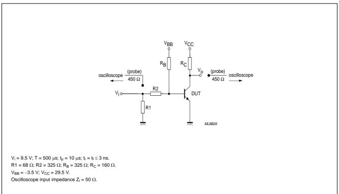
Fig.2 Test circuit for switching times.
