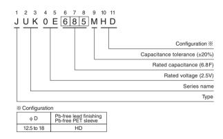
Please refer to the Guidelines for Aluminum Electrolytic Capacitors for end seal configuration information.
