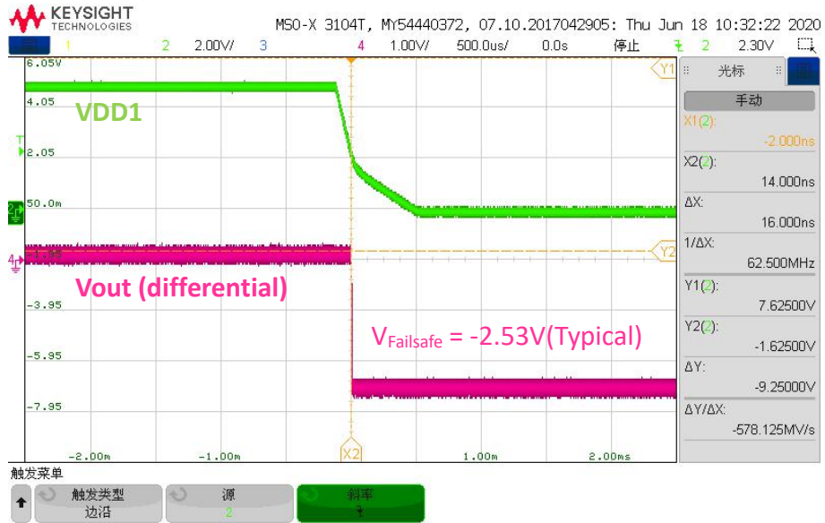
Figure 7.3 Typical Failsafe output when VDD1 undervoltage
