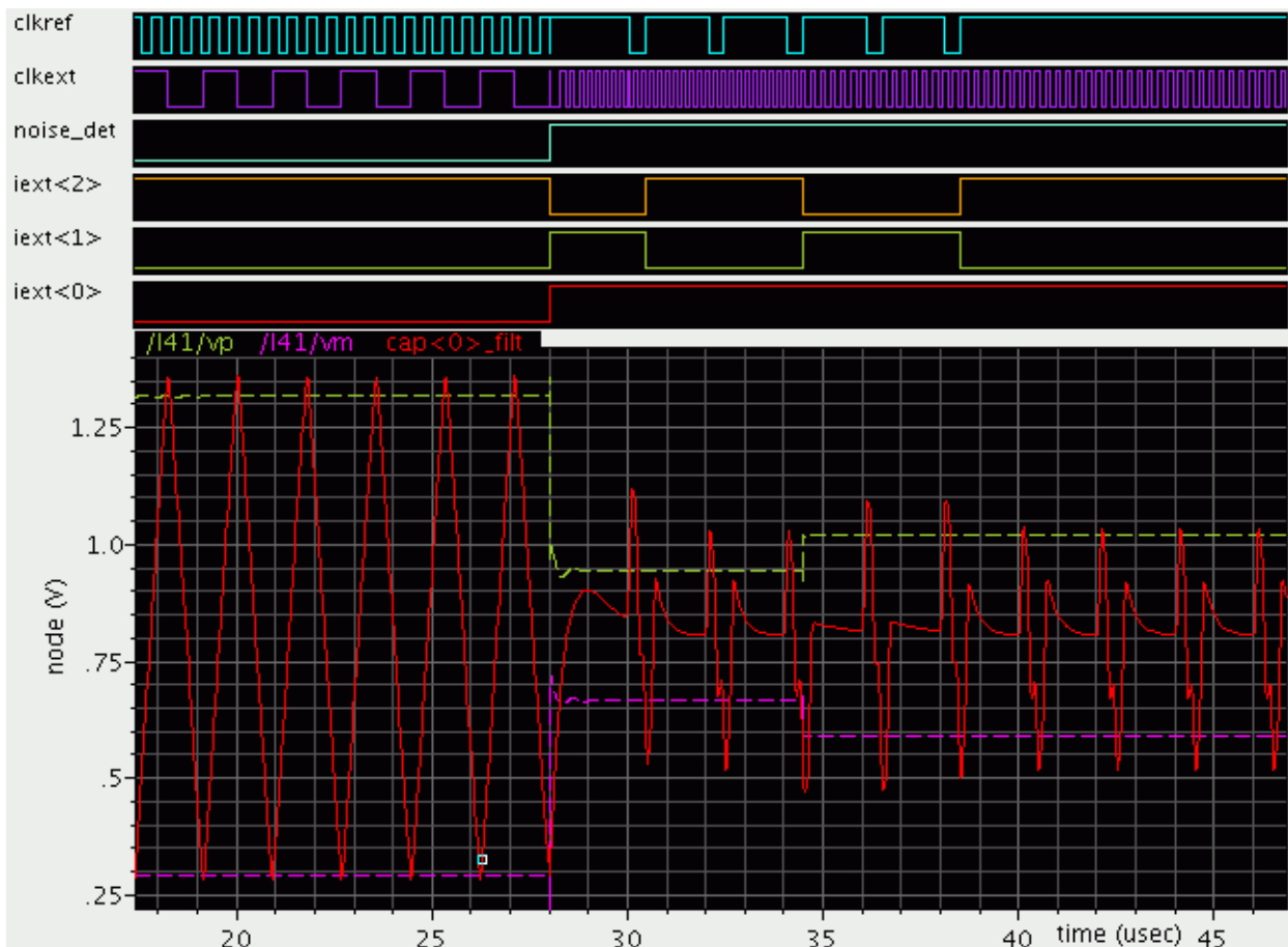
Figure 39-16. TSI noise detection mode waveform
