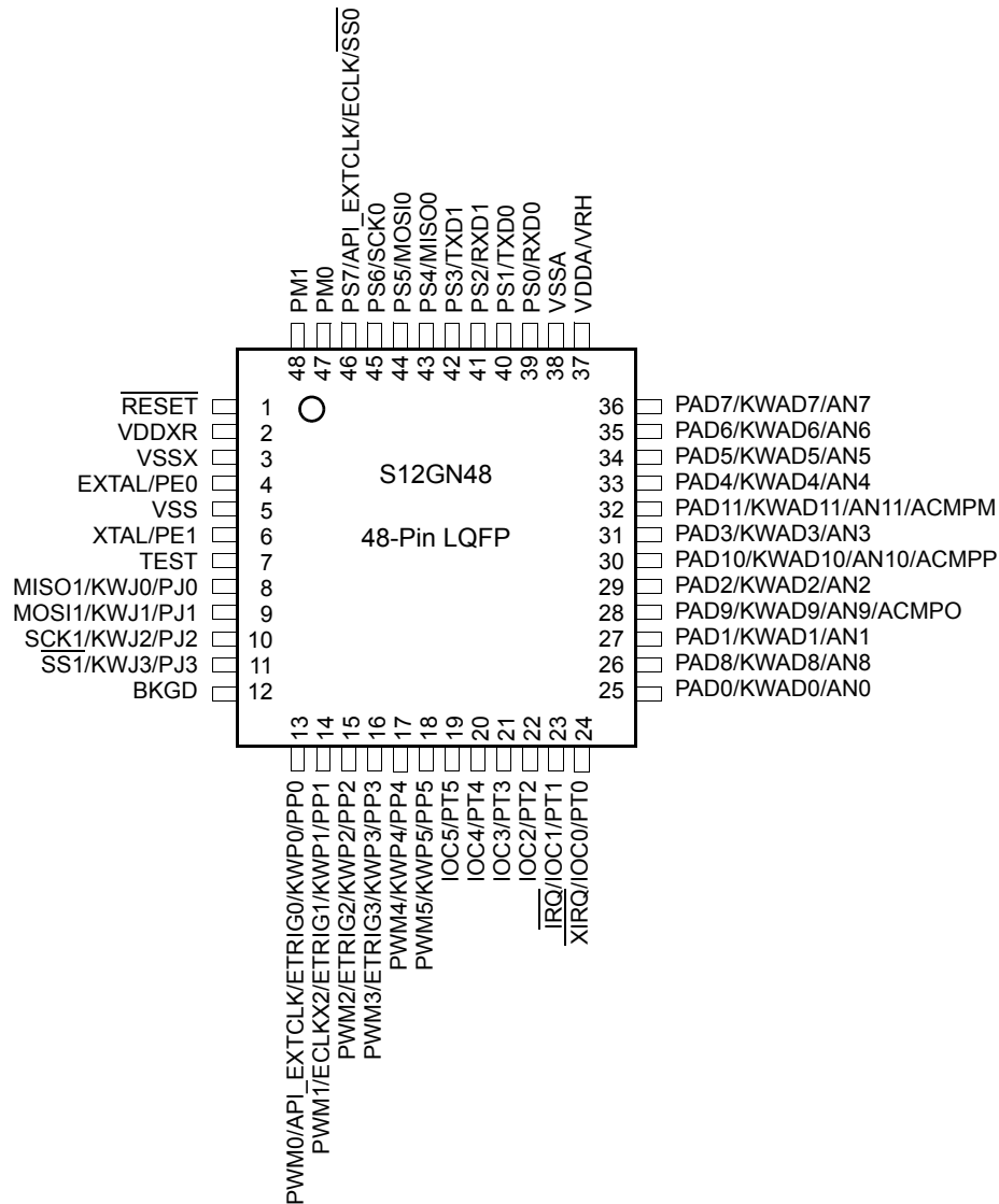
Figure 1-8. 48-Pin LQFP Pinout for S12GN48
