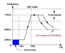
At full load conditions, there are two situations: firstly, if the system input is in low line input range, the IC operates in 65K fixed frequency CCM mode. Thus, small size transformer can be used with high power conversion efficiency. Secondly, if the system input is in high line input range, the IC operates in QR mode. In this way, high power conversion efficiency can be achieved in the universal input range when system is at full loading conditions.
