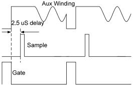
The auxiliary winding voltage is a well-defined replica of the output voltage. The OTP works by
