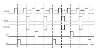
On-Bright proprietary dual function of external OTP and output OVP provides feasible and accurate detection of external OTP through NTC resistor and output OVP. The dual function is realized through time-division technology as shown in the figure.
