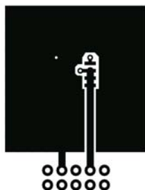
a) 50\text{ }^\circ\text{C/W} when mounted on a 1\text{ in}^2 pad of 2 oz copper.
