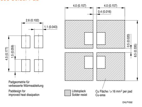
For superior solder joint connectivity results we recommend soldering under standard nitrogen atmosphere. Package not suitable for ultra sonic cleaning.
