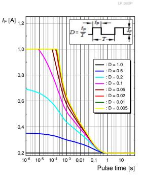
$I_{F} = f(t_{p}); D: Duty cycle$
