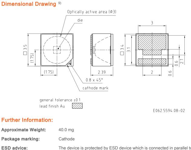
The device is protected by ESD device which is connected in parallel to the Chip.
