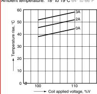
4-(2). Coil temperature rise (2 Form C 2 coil latching type) Tested sample: DS2E-ML2-DC12V Point measured: Inside the coil Ambient temperature: 20° to 21°C 68° to 70°F
