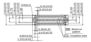
Recommended metal mask pattern Metal mask thickness: When 100 μm (Terminal opening ratio: 70%) (Metal-part opening ratio: 46%)
