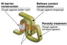
V notch and Double contact constructions
