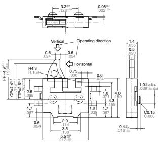
Circuit construction SPST-NO (1 Form A) Left angle
