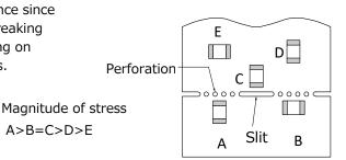
(3) The magnitude of mechanical stress applied to the Inductors when divided is in the order of push back < slit < V-groove < perforation.
