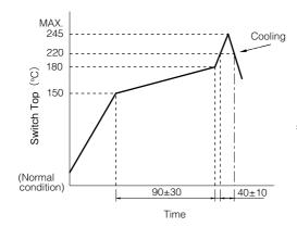
\*Reflow temperature may vary by location even in the same reflow condition. Please check the reflow temperature at terminals and at the top of a switch to make sure the both temperatures are within the specification. If even one of them is out of the specifications, please adjust.
