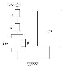
Temperature Compensation (RF circuit)
