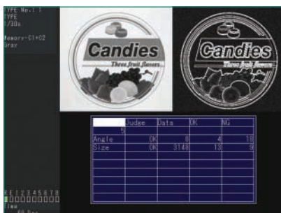
Simultaneous image display from two cameras (This shows an image processed with gray scale and binary differentiation.)
