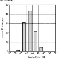
Measuring conditions Sample: CR2-12 V, 50 pcs. Equipment setting: "A" weighted, Fast, Max. hold Coil voltage: 12V DC Coil connection device: Diode Background noise: Approx. 20dB
