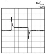
Sample: CR2-12V, 3pcs Brake current: 22A, power window motor actual load (lock condition) Tested voltage: 14V DC Switching frequency: (ON:OFF = 0.5s:9.5s) Ambient temperature: Room temperature
