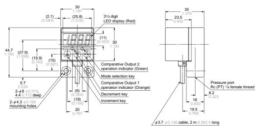
**DIMENSIONS (Unit: mm in)** The CAD data in the dimensions can be downloaded from the SUNX website: http://www.sunx.co.jp/
